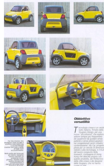
The MyCar quadricycle is quickly transformed into a hard top car or a cabriolet thanks to its structure of thermoplastic reinforced steel tubes. These structures make up most of the vehicle's weight (it is 70% recyclable).
