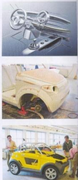
Above: The full-scale chassis model and the performance prototype under development. The quadricycle was designed by Innovech in Hong Kong in partnership with Giugiaro.
